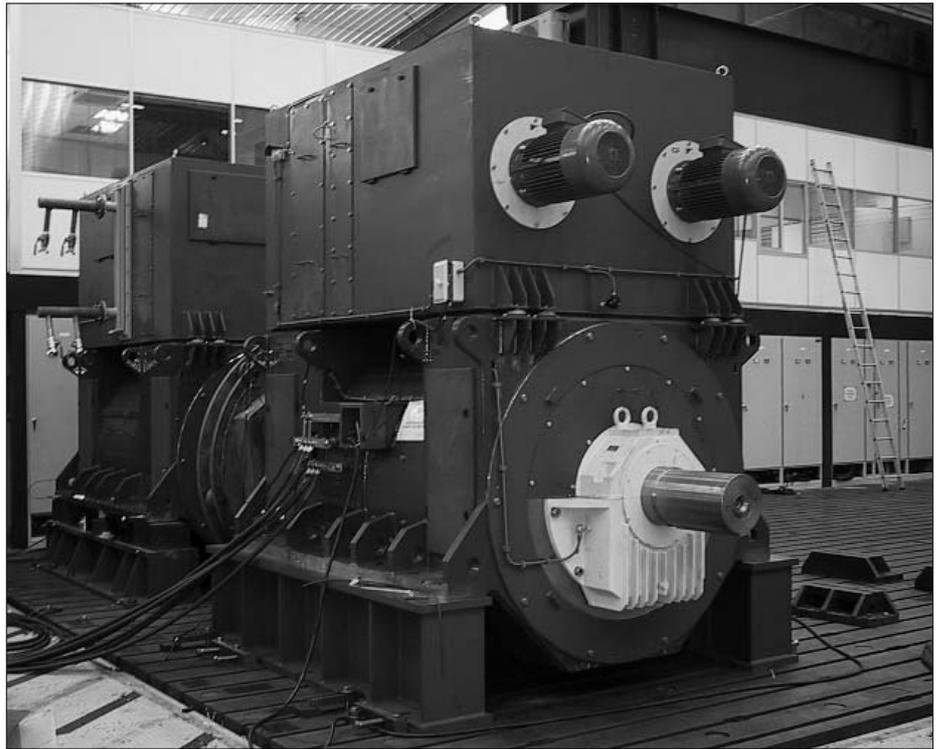
One of the two 1,500 kW low-noise Indar DC propulsion motors in tandem
